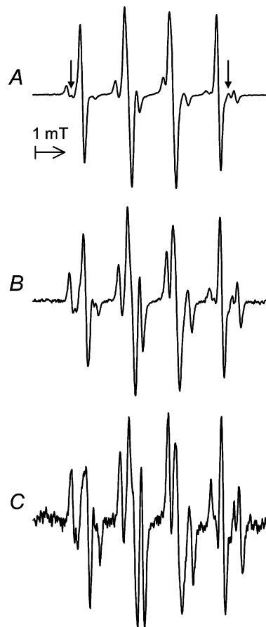
Figure 3. Spectra obtained following the reaction of 1 mM \text{CuCl}_2 with 20 mM t\text{BuOOH} in 0.1 M Tris buffer (pH 7.4) containing 4 mM Gly-Gly-Gly and DMPO at the following concentrations: (A) 400 mM, (B) 100 mM, and (C) 50 mM. The spectra B and C are shown expanded in the y-axis 5- and 25-fold, respectively, relative to spectrum A. The arrows in spectrum A indicate the outermost lines of an adduct believed to result from the trapping of a radical derived from the peptide.
